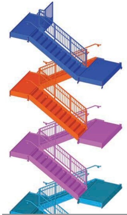
A screenshot of BIM mode of McGregor Stair System created using Tekla. Tekla is used to detail all McGregor Stairs in-house.
